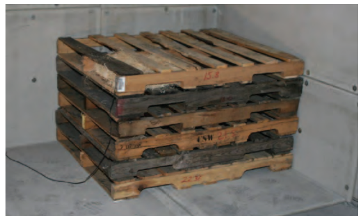
Figure A-2. Pallets and Excelsior Ignition Source Used as a Fuel Source
