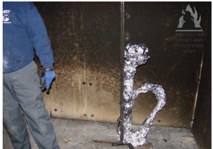
Figure A-4: Heat Flux Gauge with Radiation Shielding
